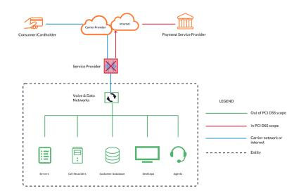
Diagram of a secure contact center.
