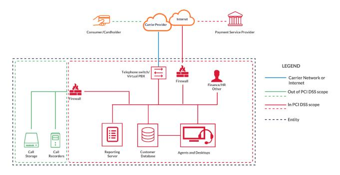
Diagram of pause and resume call recording and PCI DSS scope.
